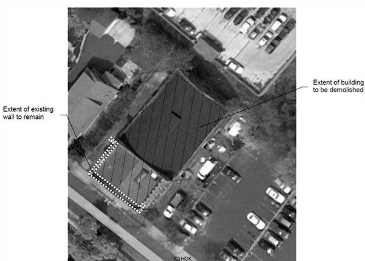
Figure 3 - Existing Structure to Remain
